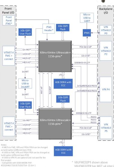
V6UFMC02P1 shown above V6UFMC02P2 has MGT x4 inter-FPGA and additional MGT x4 to P2 and P5
